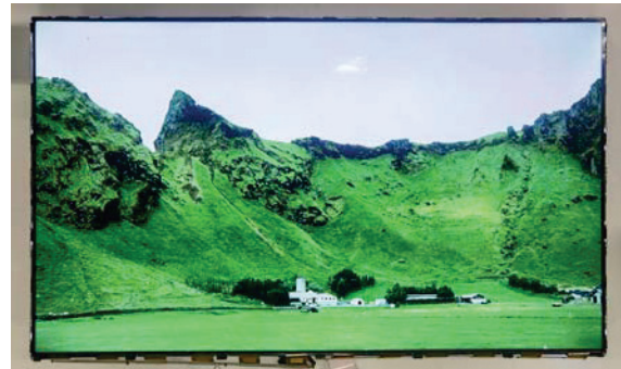
Fig.8 50 inch UHD 120Hz TFT-LCD panel with the proposed integrated gate driver GOA circuit using 4-mask a-Si TFT
