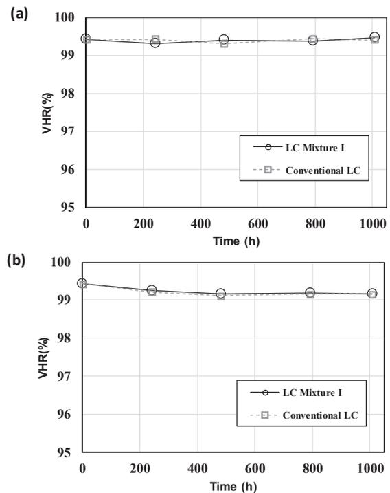
**Fig. 5** VHR as a function of aging time for (a) LED backlight exposure and (b) storage in a 70 °C oven.
