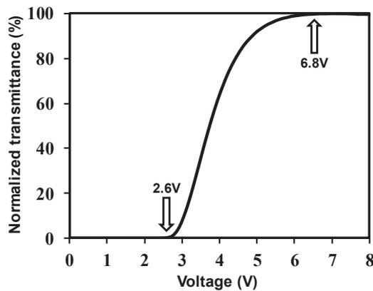
**Fig. 4** V-T curve of the PSVA Cell I.
