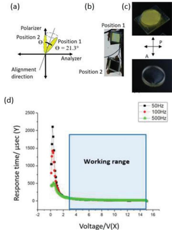
Fig. 3 (a) Schematics of the orientation of the FLC molecules during switching (b) The bright and dark states of the FLC cell which corresponds to position 1 and position 2 of the FLC molecules (c) The LC lens under crossed polarizers. The bright state is when the alignment layer is at 45° and the dark state is due to the alignment direction being parallel to the optic axis of the polarizer (d) The response time of the FLC cell as a function of voltage
