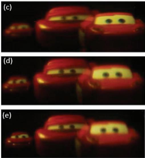
Fig. 4 (a) The FLC, lens and polarizer combination being used in the study. (b) Using the same combination, eight focusses can access as shown in the truth table. Three objects have been placed at distances of 1.2m, 1.9m and 5m. (c) Object placed at 1.2m in focus. (d) Object placed at 1.9m in focus. (e) Object placed at 5m in focus.
