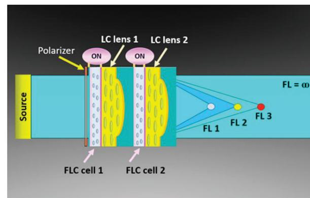
Fig. 1. Proposed structure consisting of a FLC cell and LC lens. The schematics show two such units, along with a polarizer, and four focal lengths (FLs) generated by it.
