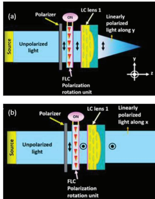
Fig. 5 (a) The focused state when the polarization direction is along the optic axis of the LC molecules ( $n_e$ ) in the lens. (b) The defocused state when the polarization direction is perpendicular to the optic axis of the LC molecules in the lens ( $n_o$ ).
