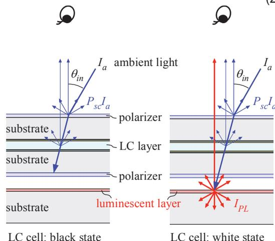
**Fig. 1 Ambient light is utilized for displaying an image by stacking an LC cell on a luminescent layer.**
