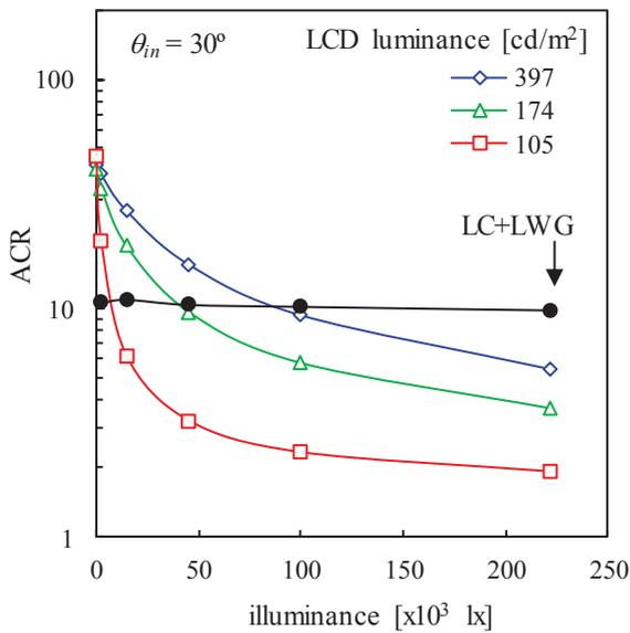
**Fig. 5 Comparison of the proposed configuration (LC cell on LWG) and a transmissive LCD.**
