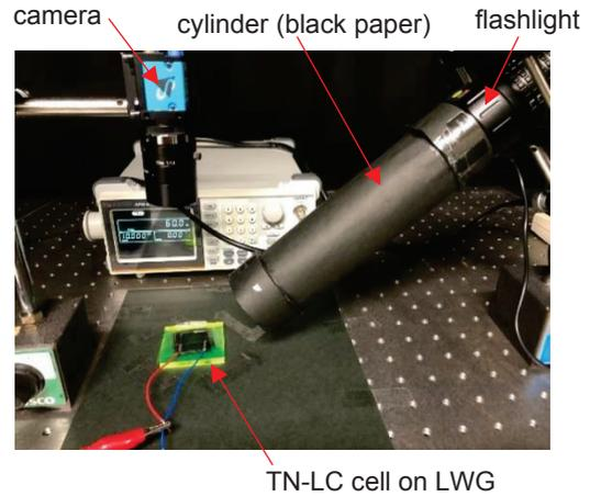
**Fig. 6 ACR measurement under the illumination with a narrower angular range.**
