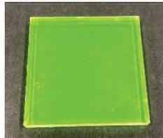
Fig. 2 Photograph of an LWG taken under room light.
