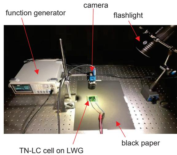
Fig. 3 Setup for the ACR measurement.
