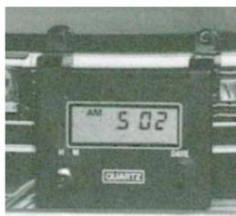
Fig. 1 The world's first LCD clock for automotive
