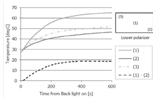
**Fig. 9 Temperature of lower polarizer 3 position after turning on the backlight**
