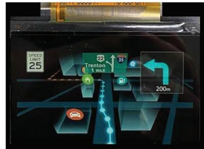
Fig. 3 Example of LCD for HUD
