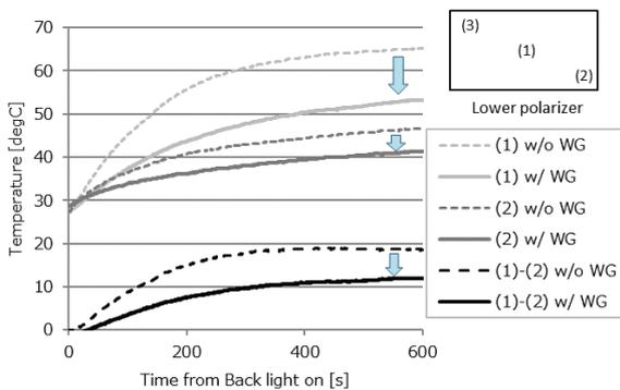
**Fig. 11 Temperature of lower polarizer with and without WG after turning on the backlight**
