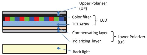
Fig. 5 Configuration of LCD and polarizer
