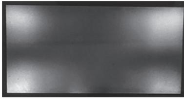
Fig. 4 Light Leakage with HUD backlight
