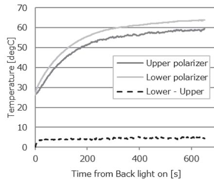
**Fig. 8 Temperature of upper and lower polarizer after turning on the backlight**
