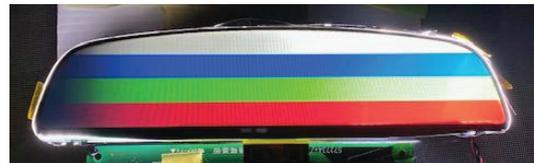
Fig. 2 Example of mirror shaped LCD
