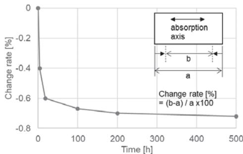
**Fig. 7 Change rate of polarizer length in absorption axis after 105degC storage time**
