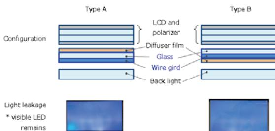
**Fig. 10 Configuration of wire grid and light leakage**
