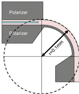
Figure 5. Cross-sectional view of polarizer film with a radius of curvature of 0.1 mm.
