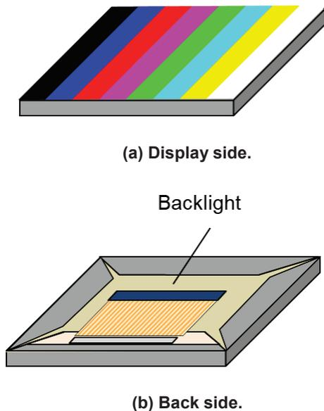
Figure 3. Sheet LCD after bending along the backlight frame.
