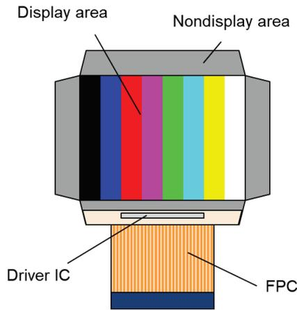
Figure 2. Sheet LCD before bending
