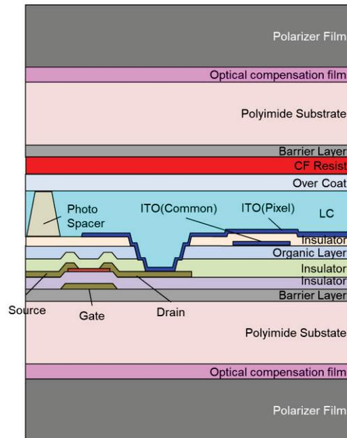
Figure 1. Cross-sectional structure of a sheet LCD.
