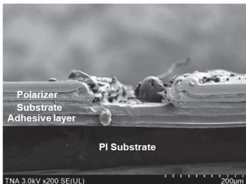
Figure 6. Cross-sectional SEM image of the lower polarizer film cut by laser.
