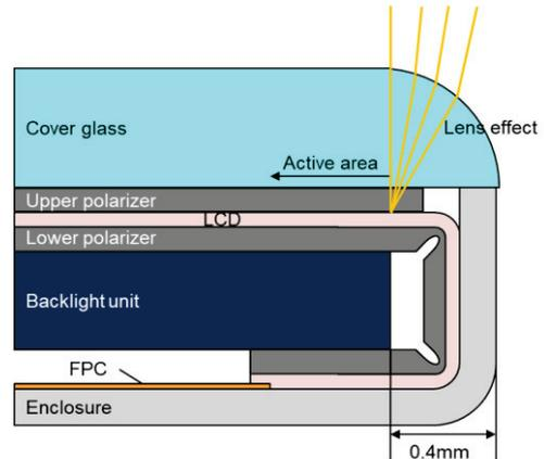
Figure 7. Cross-sectional structure of an ultra-narrow-border LCD module.
