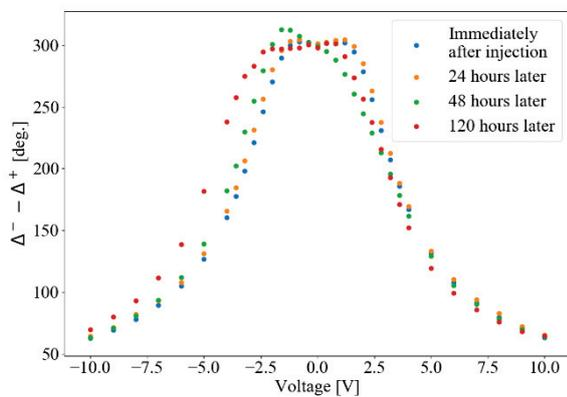
**Fig.6 Time dependence of  $\Delta^- - \Delta^+$  measurement under DC applied voltage.**
