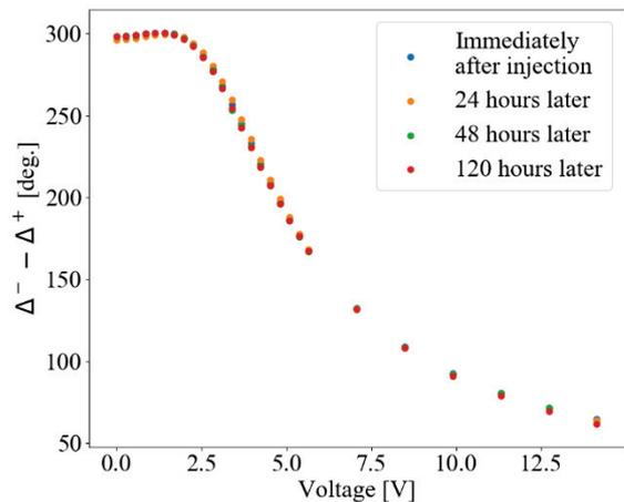
Fig.5 Time dependence of  $\Delta^- - \Delta^+$  measurement under rectangular AC applied voltage.
