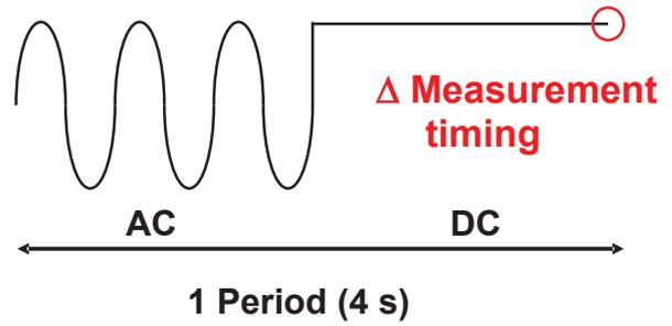
Fig.4 Timing chart of applied voltage and  $\Delta$  measurement, where 1 period is 4 s.
