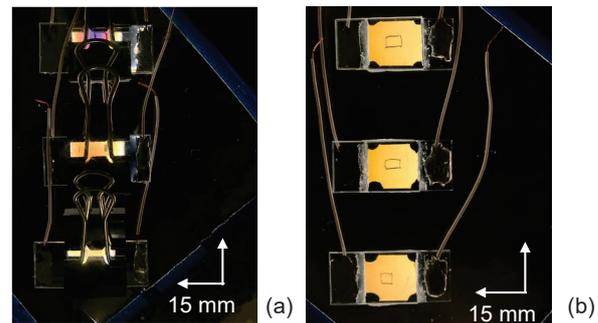
Fig.2 Photograph of sample cell under the crossed polarizer films. (a) Fixed by foldback clip. (b) Cemented by epoxy resins. The white arrow corresponds the axis of polarizer, and the length of the arrow exhibits 15 mm.
