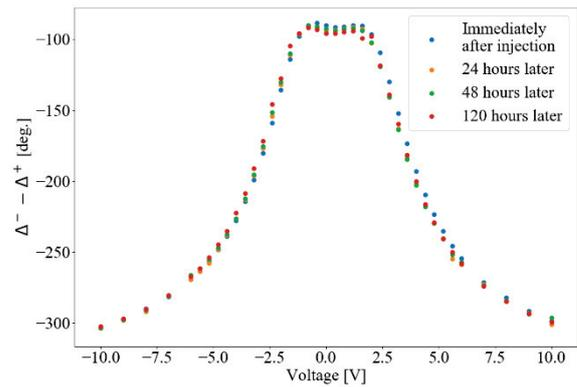
**Fig.7 Time dependence of  $\Delta^- - \Delta^+$  measurement under DC applied voltage, where the sample NLC was unsealed with epoxy resins.**
