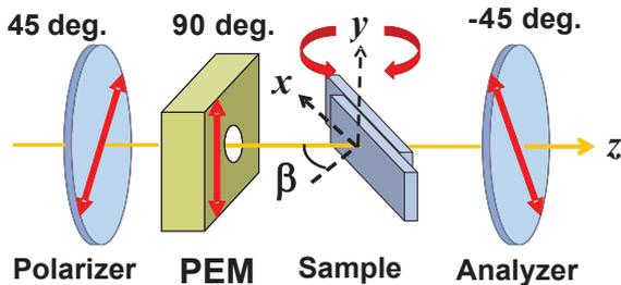
Fig.3 Transmission Ellipsometry with LC sample rotation stage.
