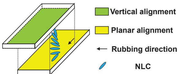
Fig.1. Schematic of the sample HAN cell.
