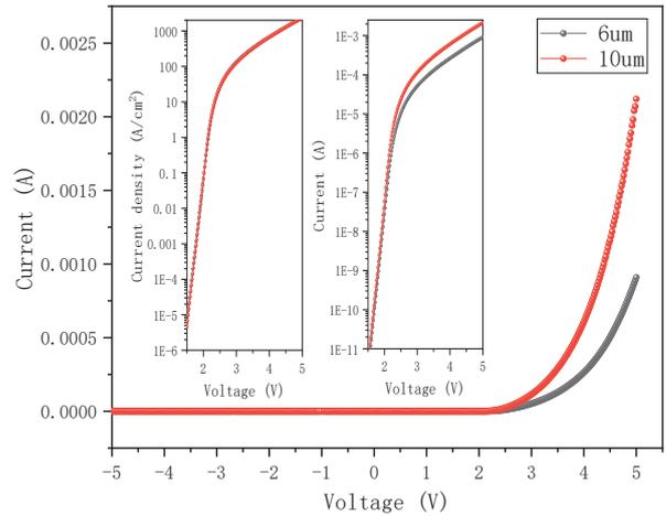
**Fig.3 The current-voltage semi-log curve with current density-voltage semi-log curve inset of device size with 6\*6.5um<sup>2</sup> and 9.5\*9.5um<sup>2</sup>.**
