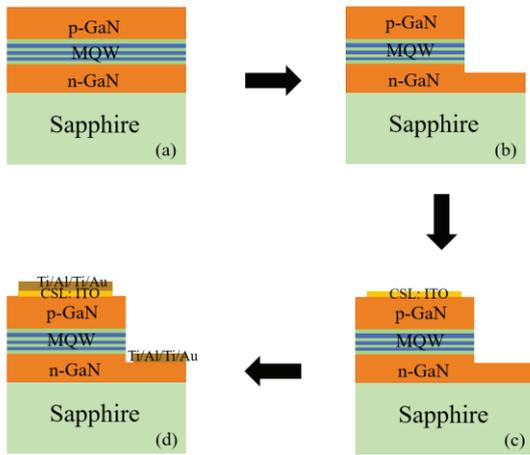
**Fig.1 Fabrication process**
