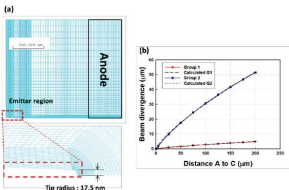
**Fig. 2 Simulation results. (a) Modeling of SOURCE 2D simulation in diode mode, (b) electron beam trajectory prediction by distance.**
