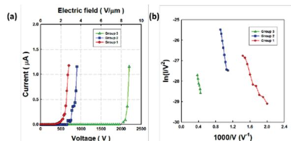
**Fig. 1 Comparison of field emission properties. (a) Field emission properties of Group 1, 2, 3, (b) F-N plot.**
