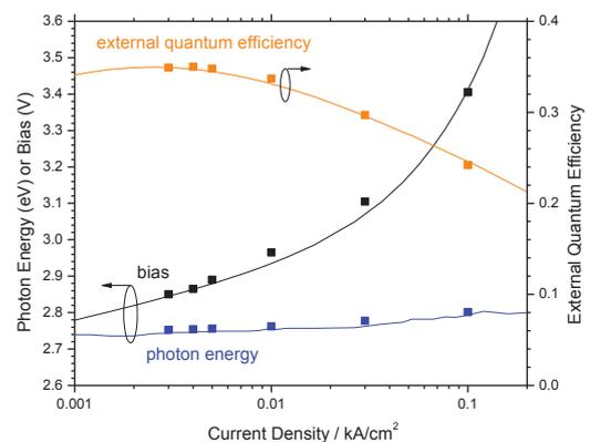
Fig. 1: Comparison of measurements (symbols) and simulations (lines) for the blue LED.
