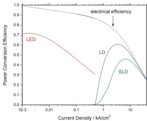
Fig. 3: Comparison of the power conversion efficiency PCE calculated for LED (red), laser (blue) and SLD (green). The top dashed line gives the electrical efficiency.
