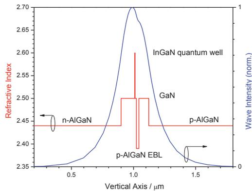
Fig. 2: Refractive index and wave intensity profiles.
