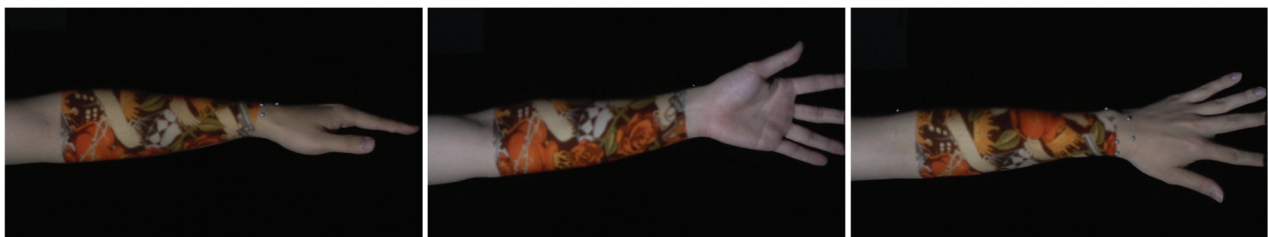
Fig. 3 High-speed human arm projection mapping with skin deformation [8]
