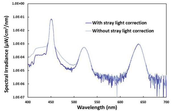
**Fig. 6 Log scale spectral irradiance of blue with and with spectral stray light correction.**
