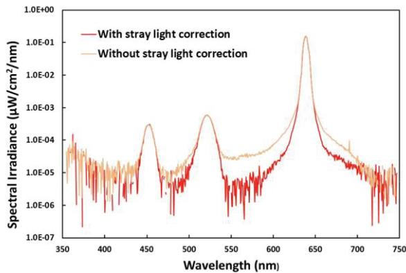
**Fig. 4 Log scale spectral irradiance of red with and with spectral stray light correction.**
