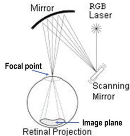
Fig. 1 Example configuration setup of a retinal projection device.
