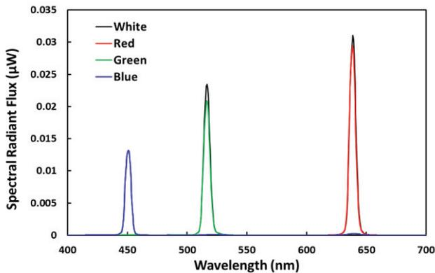
**Fig. 2 Example white, red, green, and blue spectral radiant flux of commercial retinal projection device.**
