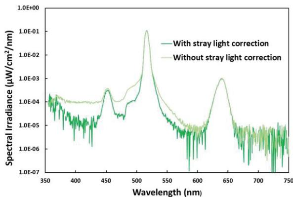
**Fig. 5 Log scale spectral irradiance of green with and with spectral stray light correction.**
