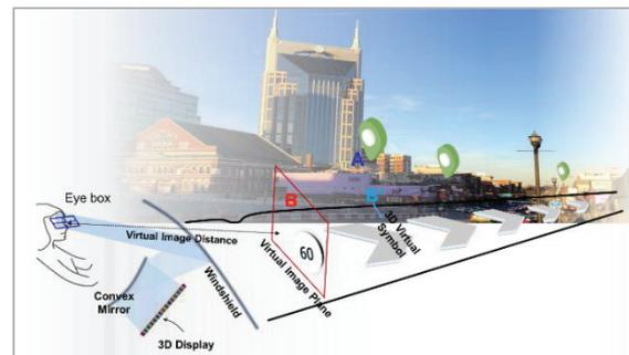
**Fig. 1 The B symbol on 2D HUD vs. the stereo B' symbol with depth information indicating the real building A on the street.**
