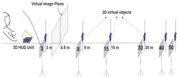
**Fig. 5 Experimental configuration for the perceived distance in 3D HUD**
