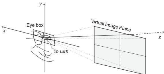
Fig. 3 The geometric relationship between an eye-box and a virtual image plane
