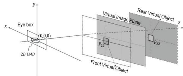
Fig. 4 Measuring condition for the 3D virtual object distance for the virtual object in the front or rear of the virtual image plane
