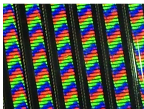
Fig. 4 Magnified image observed through lens array.
