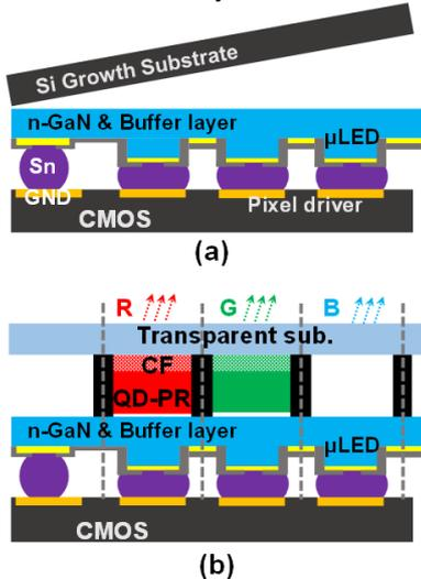
**Fig. 1 (a) Structure of the integrated blue micro-LED chip. (b) Schematic of full-color micro-display using blue micro-LEDs and Red/Green QDPR.**
