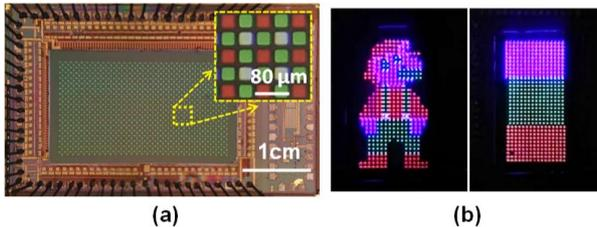
**Fig. 2 (a) 32  $\times$  18 full-color micro-display chip. Inset is a zoomed-in image of the color conversion layer. (b) Full-color images rendered on this full-color micro-display system.**
