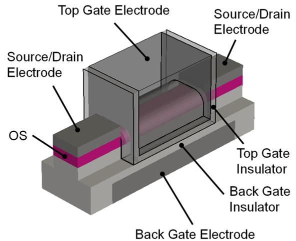
**Fig. 4 Schematic view of OSFET (W/L = 60 nm/200 nm)**
