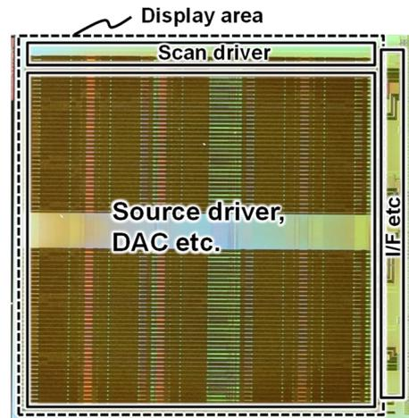
**Fig. 9 Die photograph before OSFET fabrication**
