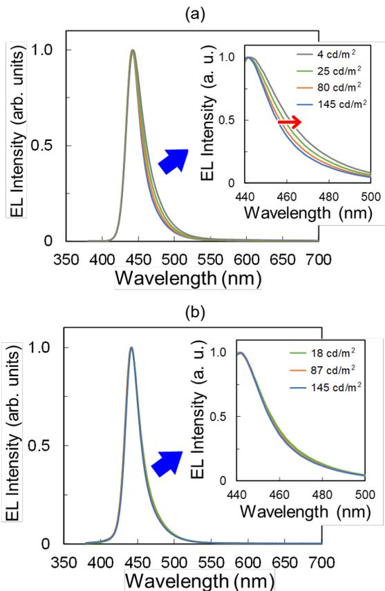
Fig. 2 EL spectra of the QD-LEDs whose EML was composed of (a) only ZnSeTe QDs and (b) the mixture of ZnSeTe QDs and ETM.
