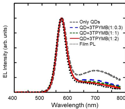
Fig. 4 The EL spectra of the QD-LEDs fabricated using AIS core/shell QDs, and the PL spectrum of the QD film.
