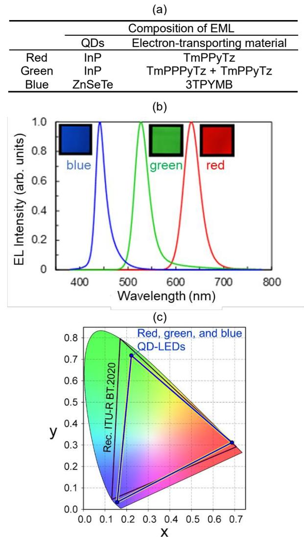
Fig. 3 (a) Composition of the EML, (b) the EL spectra, and (c) the chromaticity coordinates (CIE1931) at a luminance of  $100 \text{ cd m}^{-2}$  for the fabricated red, green, and blue QD-LEDs.
