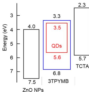
Fig. 5 Energy levels of the materials used in the QD-LEDs fabricated using AIS core/shell QDs.
