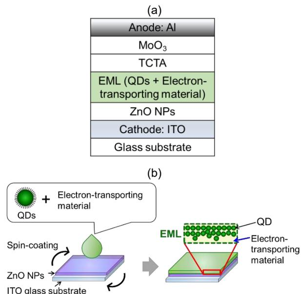
Fig. 1 (a) Device structure of the fabricated QD-LEDs and (b) the formation of an emitting layer (EML) by spin-coating a mixed solution of QDs and an electron-transporting material.
