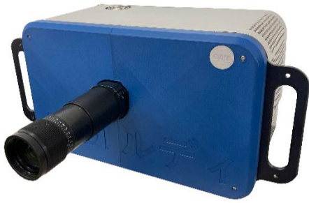
Fig. 1 Developed high-speed RGB+IR projector
