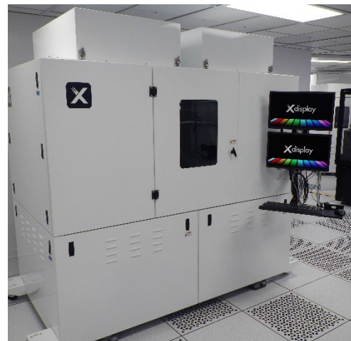
Fig. 3 Photograph of a MTP300 transfer printer with 600 mm x 800 mm stage travel.
