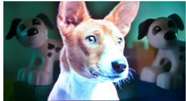
Fig. 1 Photograph of a transparent 320 x 160 70 PPI microLED display in front of toy dogs.
