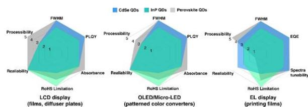
Figure 1 | The key merits between conventional QDs (CdSe and InP ) and PQDs including absorbance coefficient, FWHM, PLQYs or EQE, as well as the processibility, reliability, and RoHS limitation.
