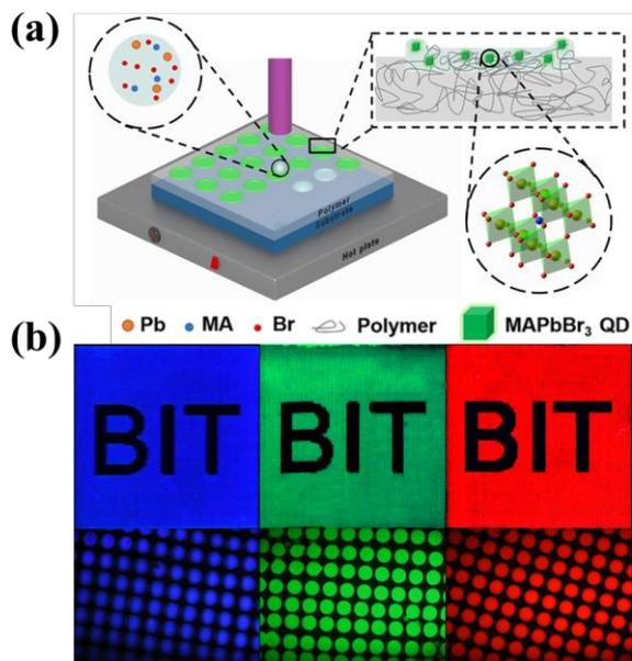
**Fig. 2** (a) Schematic diagram of the in situ inkjet printing strategy. (b) The optical images and microscopic fluorescent images of printed PQDs patterns with red, green and blue colors under UV light illuminations.
