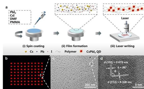
**Fig. 3** In-situ direct laser writing fabrication of patterned  $\gamma$ -CsPbI<sub>3</sub> PQDs. (a) Schematic illustration of the process of direct laser writing. (b) The resulting patterned  $\gamma$ -CsPbI<sub>3</sub> PQDs under UV-365 nm light illumination. (c) TEM image of resulting  $\gamma$ -CsPbI<sub>3</sub> PQDs obtained from direct laser writing. (d) HRTEM image of single  $\gamma$ -CsPbI<sub>3</sub> PQD.
