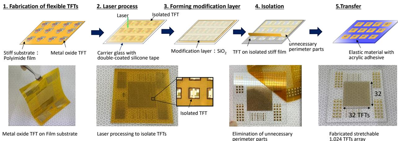
**Fig. 2. The fabrication process of stretchable metal oxide TFTs array with acrylic adhesives to obtain reliable stretchability. Processes are consisted of mainly 3 steps: i) fabrication of flexible TFTs array, ii) isolation process of TFTs, iii) transfer process to the stretchable substrate.**
