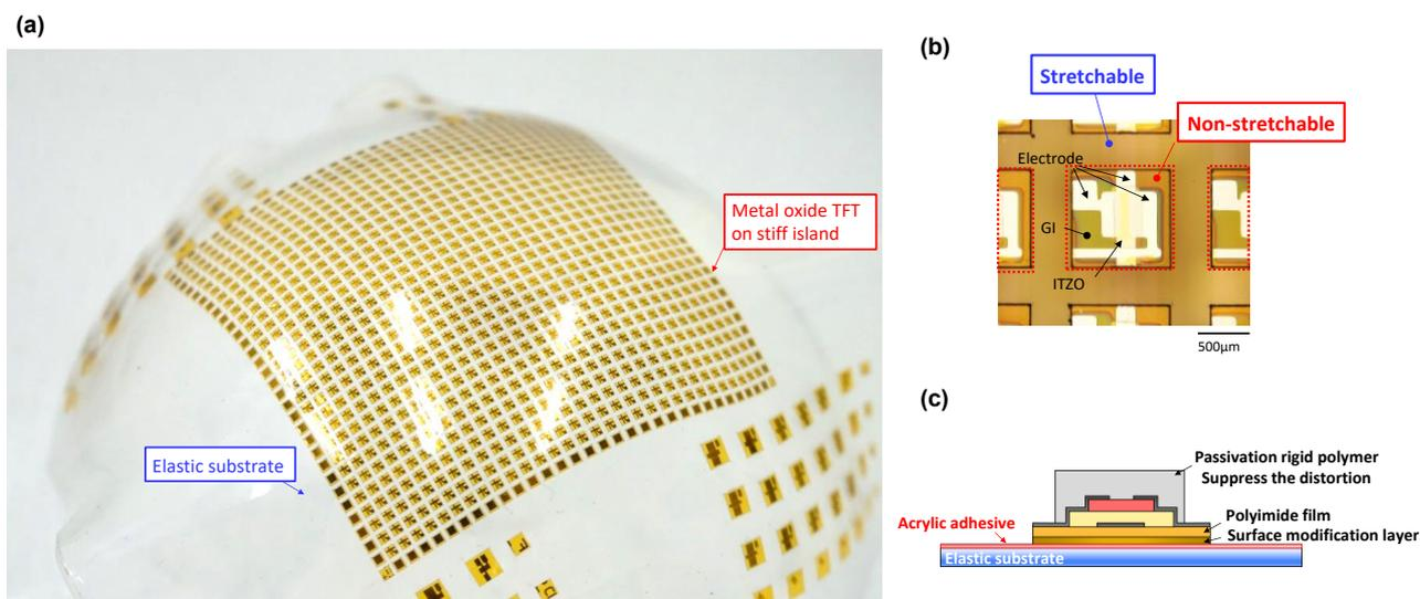
**Fig.3. (a) A photograph of fabricated dome-shape stretchable metal oxide TFTs array with acrylic adhesive and (b) Magnified image of metal oxide TFT, and (c) Schematic of the TFT structure with acrylic adhesive and modification layer to achieve better integration between polyimide film and elastic substrate.**
