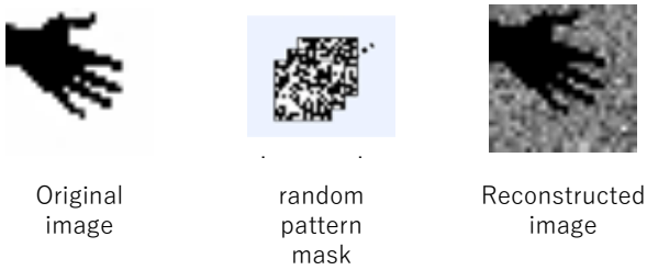
Fig. 4 Reconstructed image with single pixel imaging by use of 10000 random pattern masks.
