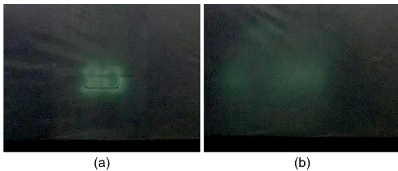
Fig. 15 Result of placing the screen at the forming position of the aerial image with a PET bottle. A bottle touches (a) the beam splitter and (b) the light source.
