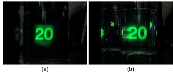
Fig. 12 Result of using a cylinder as the key. A cylinder touches (a) the beam splitter and (b) the light source.
