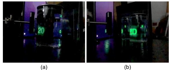
Fig. 13 Lateral viewing angle in a cylinder. (a) touches the beam splitter is wider than (b) touches the light source.
