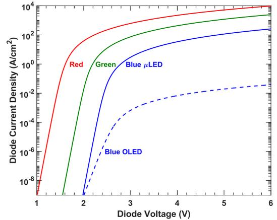
**Fig. 4.**  $I - V$  curves for red, green, and blue  $\mu$ LEDs (this work) and a modern blue OLED [Ref. 20]. There exists a fundamental gap between the current carrying capability of inorganic  $\mu$ LEDs and OLEDs ( $\sim 10,000\times$ ). The lines are best fits to experimental data (not shown here for clarity).
