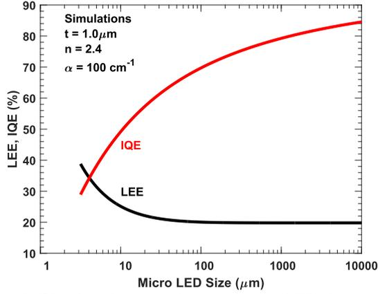
**Fig. 2.** Simulated *LEE* and *IQE* versus  $\mu$ LED size. *IQE* degrades with decreasing the  $\mu$ LED size, and the increase in *LEE* with smaller  $\mu$ LED size is not enough to compensate for the *IQE* degradation, resulting in degraded *EQE* at smaller LEDs as shown in [16-19].
