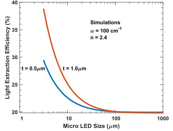
**Fig. 1.** Simulated light extraction efficiency ( $LEE$ ) for LEDs with various lateral dimensions using equations (1)-(15). The thickness of the  $\mu\text{LED}$   $t$  is set to 0.5 and 1.0  $\mu\text{m}$ . The  $LEE$  increases as the size of the  $\mu\text{LED}$  is reduced below  $\sim 50$   $\mu\text{m}$ .
