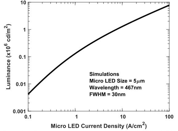
**Fig. 3.** Theoretical  $L - J$  curve for GaN  $\mu$ LEDs showing 1-10 million nits is possible.
