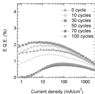
**Fig. 1.** EQE of the inkjet-printed QLEDs with varying the number of ALD cycles.
