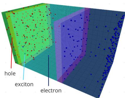
**Fig. 2 Visualization of a Bumblebee OLED device simulation - Digital twin of the device.** Holes, electrons and excitons are indicated. Bumblebee simulates charge transport and excitonic processes on each molecular site in 3D. The interplay among all these processes is simulated in time.
