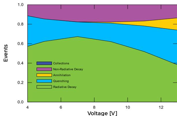
**Fig. 6 Excitonic events contributing to the device efficiency and losses at each voltage.**
