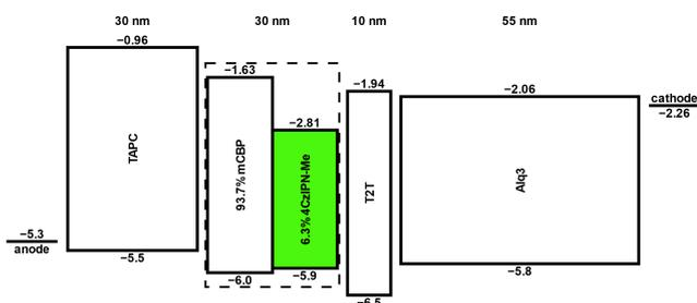
**Fig. 3 Energy diagram of the simulated stack.**
