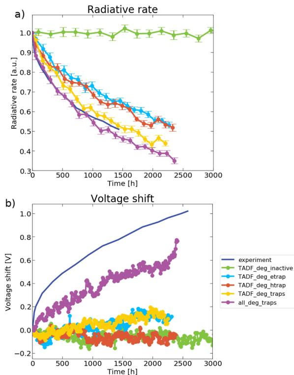
**Fig. 7 Lifetime prediction for different degradation scenarios.** a) decay in radiative rate due to degradation and b) voltage shift during degradation. The degradation products properties are varied.
