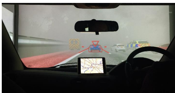
Fig. 2 HUD1: AR HUD for navigation/guidance.
