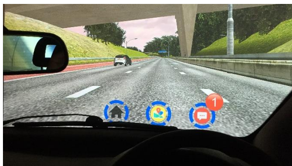
Fig. 3 HUD2: AR and gesture recognition HUD for infotainment.
