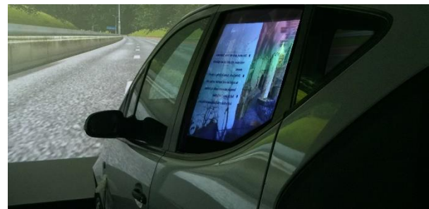
Fig. 4 HUD3: AR and gesture recognition HUD for passenger infotainment and driver's HUD interface for navigation.
