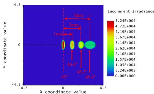
**Figure 8 – Calculated Spot Locations at Focal Plane versus Rotating Tilted Mirror Angles**
