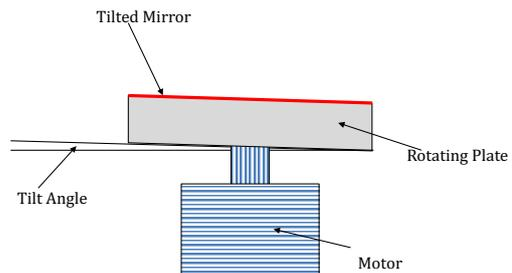
**Figure 6 – A Tilted Rotating Mirror**
