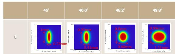
**Figure 9 – Calculated Spot Dimensions at Focal Plane versus Rotating Tilted Mirror Angles**
