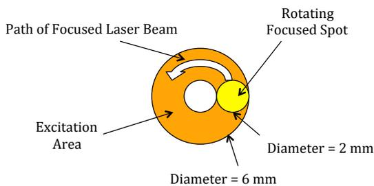
**Figure 3 – Locus of the Focus Laser Spot on the Phosphor Plate**
