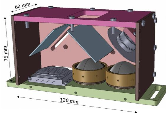
**Figure 10 – Prototype Design of the Scanning Focus Beam Static Phosphor System with White Light Output**
