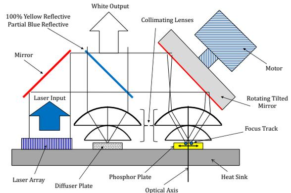
**Figure 4 – Scanning Focus Beam Static Phosphor System with White Light Output**
