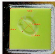
**Figure 7 – Locus of the Damaged Laser Spot on the Phosphor Plate**
