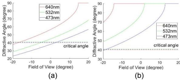
**Fig. 5 The diffractive angle simulations of (a) DWE 1 (b) DWE 2 with each LASER were utilized to expect the maximum FOV.**
