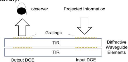
Fig. 1 The schematic diagram described the full-color AR display composed of two diffractive waveguide elements.
