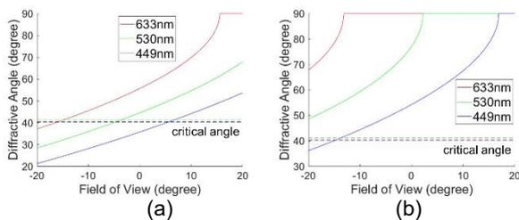
**Fig. 2 The relationship between incident angle and propagating angle of (a) DWE 1 and (b) DWE 2 was utilized to expect the FOV with different wavelengths backlight.**
