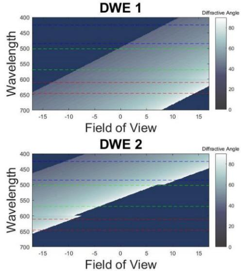
**Fig. 8 The relationship between incident angle and propagating angle of DWEs was utilized to expect the FOV with each spectrum of the LED backlight.**
