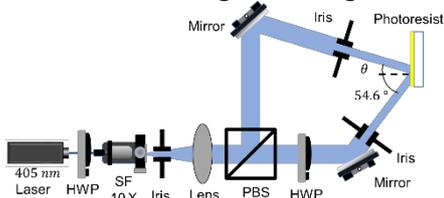
**Fig. 3 The recording system for DWE. HWP: half-wave plate; PBS: polarized beam splitter; SF: spatial filter.**
