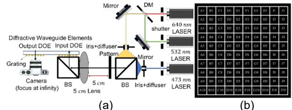
**Fig. 4 The final image with LASER backlight was recorded by (a) the experimental setup with (b) the target pattern. BS: beam splitter; DM: dichroic mirror.**
