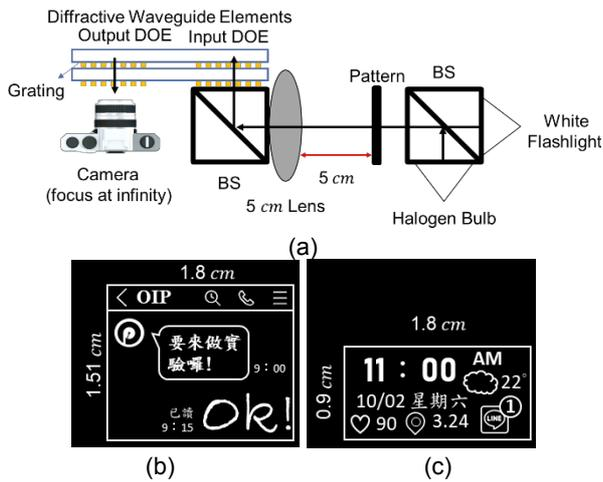
**Fig. 9** The (a) full-color display system employed the (b) pattern 1; (c) pattern 2 to confirm the full-color FOV that this system can display.
