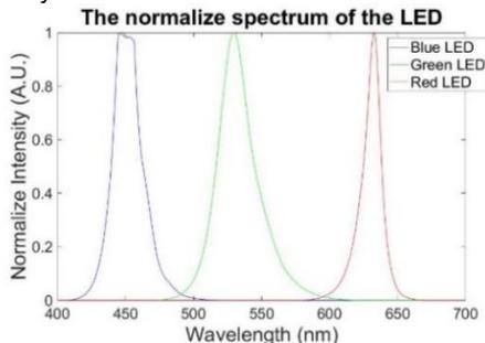
**Fig. 7 The spectrum of the red, green and blue LED.**
