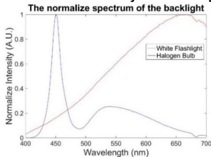
**Fig. 10** The spectrum of the full-color display based on the white flashlight and the halogen bulb.
