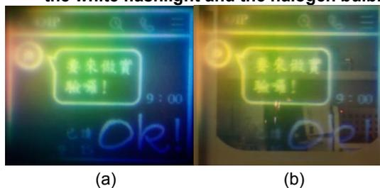
**Fig. 11** The full-color image for the larger pattern was recorded in (a) dark room; (b) bright room.
