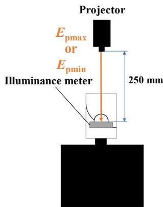
Figure 3. Method of measuring projector illuminance
