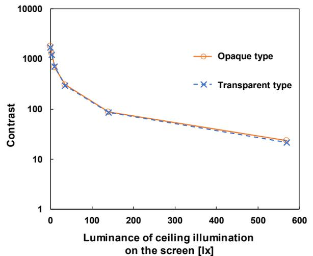
Figure 8. Ceiling illumination dependence of 3D image contrast
