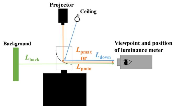
Figure 5. Parameters for determining contrast of the display in this 3D system
