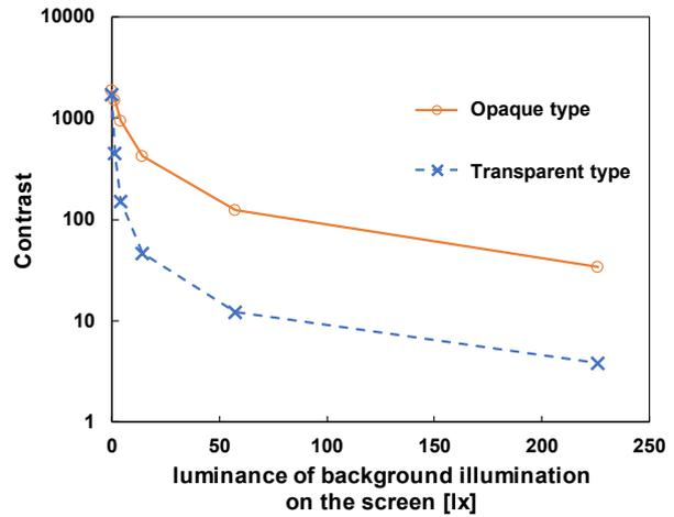
Figure 6. Background illumination dependence of 3D image contrast
