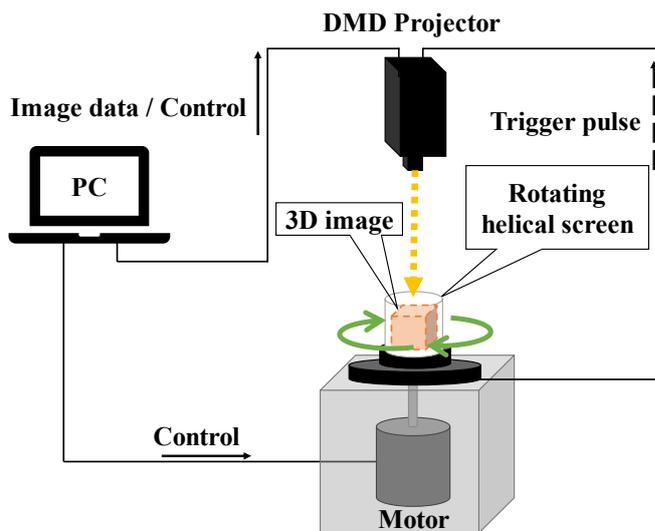
Figure 1. Arrangement of the proposed 3D display system
