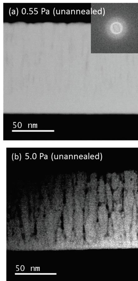
Fig. 3. HAADF-STEM images for (a) high-density film and (b) low-density film prepared by different deposition pressure.
