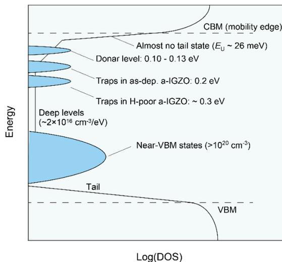
Fig. 1 Electronic structure of a-IGZO with subgap defects reported so far
