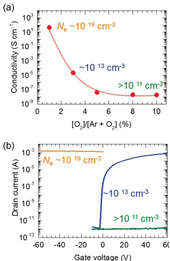
Fig. 2. (a) Conductivity change as a function of oxygen flow ratio ( $R_{O_2}$ ). (b) Transfer curves of unannealed a-IGZO TFTs corresponding to  $R_{O_2} = 1, 3,$  and  $8\%$  in (a).
