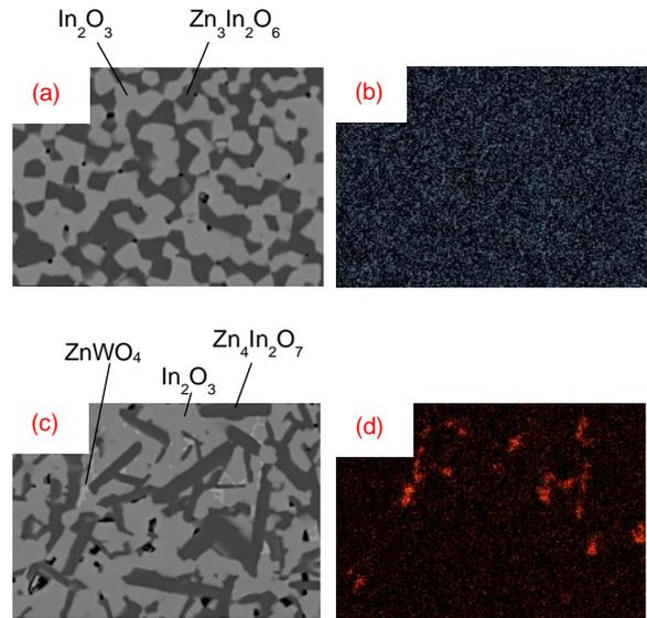
Fig. 2 SEM-BSE image of In-Zn-O-Ta (a) and In-Zn-O-W (c). EDS Ta mapping of In-Zn-O-Ta (b), and W mapping of In-Zn-O-W (d) sputtering targets
