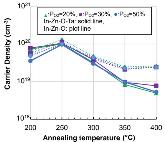
Fig. 3 Hall-measurement results of In-Zn-O-Ta (solid) and In-Zn-O (plot) films under various sputtering and annealing conditions
