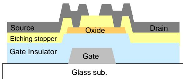
Fig. 1 TFT configuration
