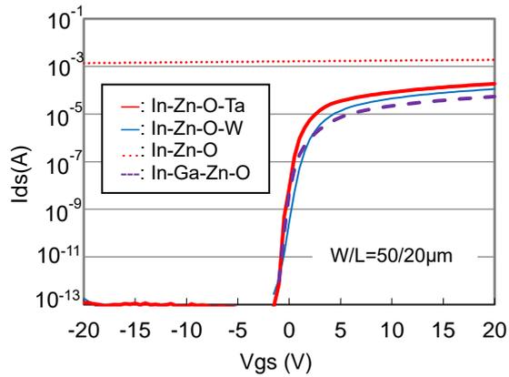
**Fig. 4** Transfer curves of In-Zn-O-Ta (red solid), In-Zn-O-W (blue solid), In-Zn-O (red plot), and In-Ga-Zn-O (violet dashed) TFTs
