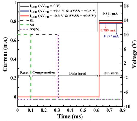
Fig. 3. Driving currents for mini-LED with  $V_{TH}$  variations of  $\pm 0.3$  V and  $V_{SS}$  I-R rise of 0.5 V.
