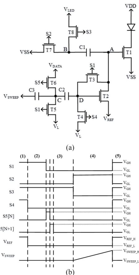
Fig. 1. (a) Proposed mini-LED pixel circuit for backlight and (b) timing diagram.
