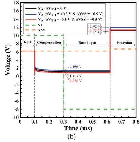
Fig. 2. Transient waveforms of (a) node D and (b) node A with V<sub>TH</sub> variations of  $\pm 0.3$  V and V<sub>SS</sub> I-R rise of 0.5 V.
