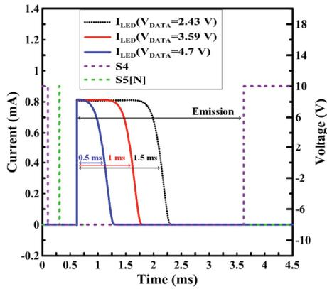
Fig. 4. Transient waveforms of driving currents at low, medium, and high gray levels.
