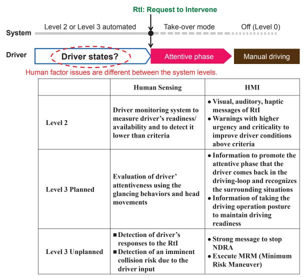
Fig. 2 Human sensing and HMI in level2, level 3 planned, and level 3 unplanned transition
