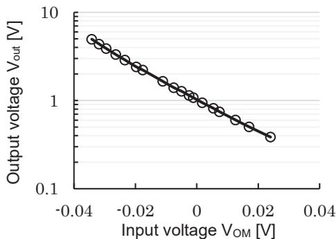
**Fig. 10** Converting characteristic of exponential converting circuit
