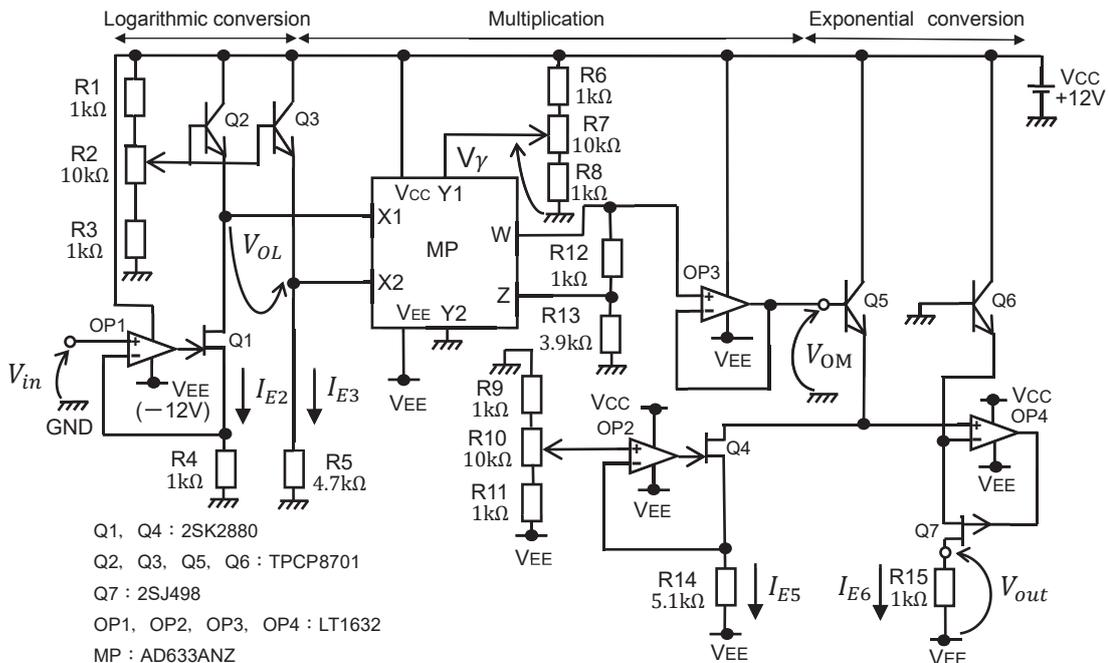
Fig. 8 Circuit configuration of the Gamma correction
