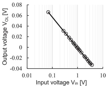
**Fig. 9** Converting characteristic of logarithmic converting circuit
