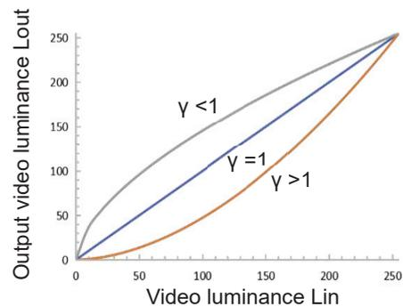
Fig. 6 Gamma correction characteristics in proposed circuit
