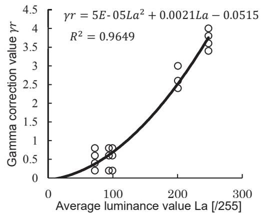
Fig. 5 Average luminance value-the Optimal gamma correction value characteristics
