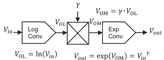
Fig. 7 Block diagram of gamma correction circuit
