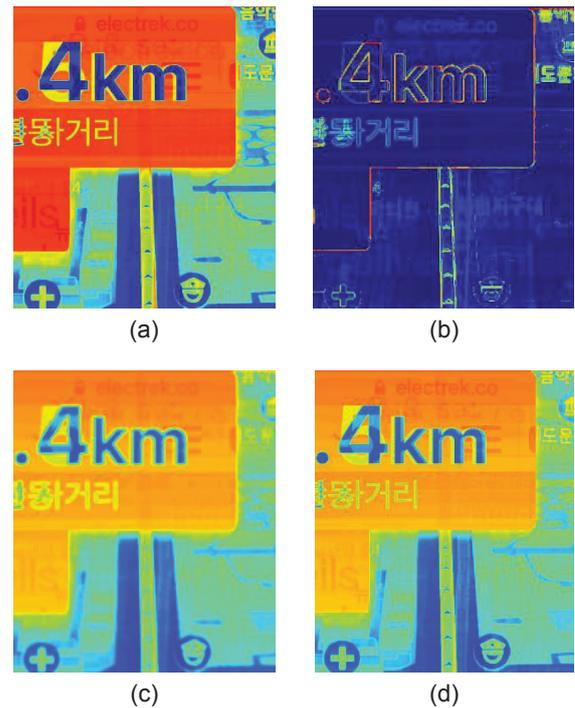
Fig. 4 Example of paired data set (a) simulated degradation map based on degradation model, (b) detail layer accumulated map, (c) simulated optical imaging data, (d) ground truth
