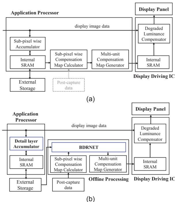
Fig. 1 Overall block diagram of burn-in compensation on the mobile system proposed in [5] (a) and in this paper (b)
