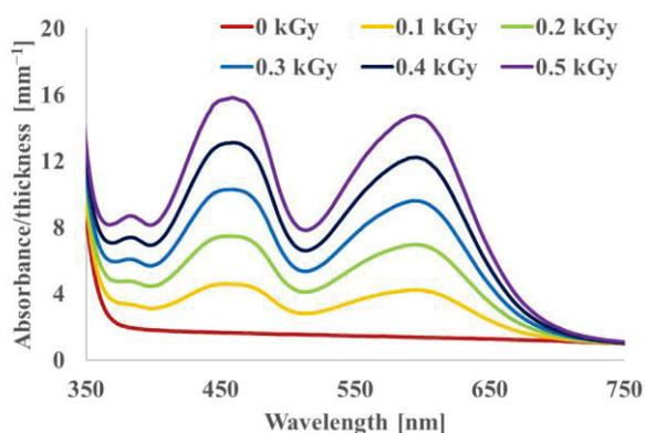
Fig. 4. Absorption spectra of PVC film containing 1 wt% Black400 before and after X-ray irradiation (0–0.5 kGy).
