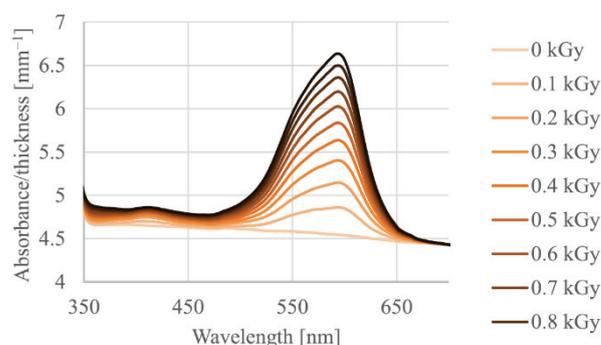
Fig. 1. absorption spectra of PVC films containing 1 wt% LCV before and after X-ray irradiation up to 0.8 kGy. Copyright (2020) The Japan Society of Applied Physics [2].
