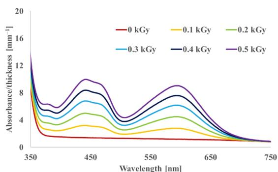
Fig. 3. Absorption spectra of PVC film containing 1 wt% Black100 before and after X-ray irradiation (0–0.5 kGy).
