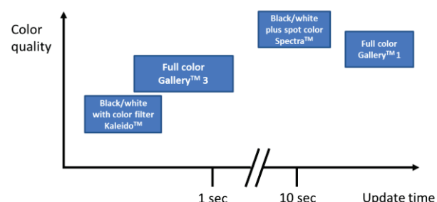
Figure 1. Summary of E Ink's color electrophoretic display technologies
