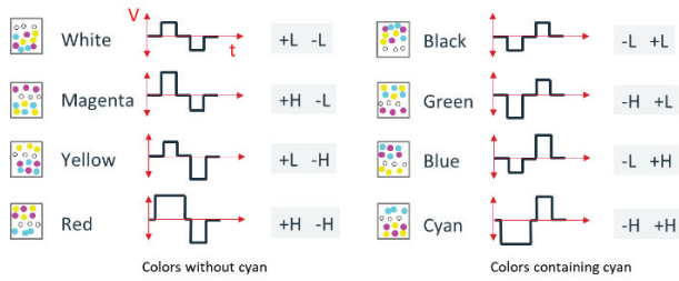
Figure 4. Representation of the voltage levels in dipole pulses required to form the 8 primary colors in an E Ink Gallery™ 3 display
