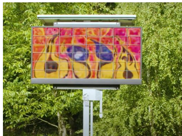
Fig 4. Etulipa full-color matrix EWD display with a still image of a displayed video. A solar panel is mounted on top of the display for power generation. With a storage battery in the trailer (not seen on the photo) the system runs forever on solar power.
