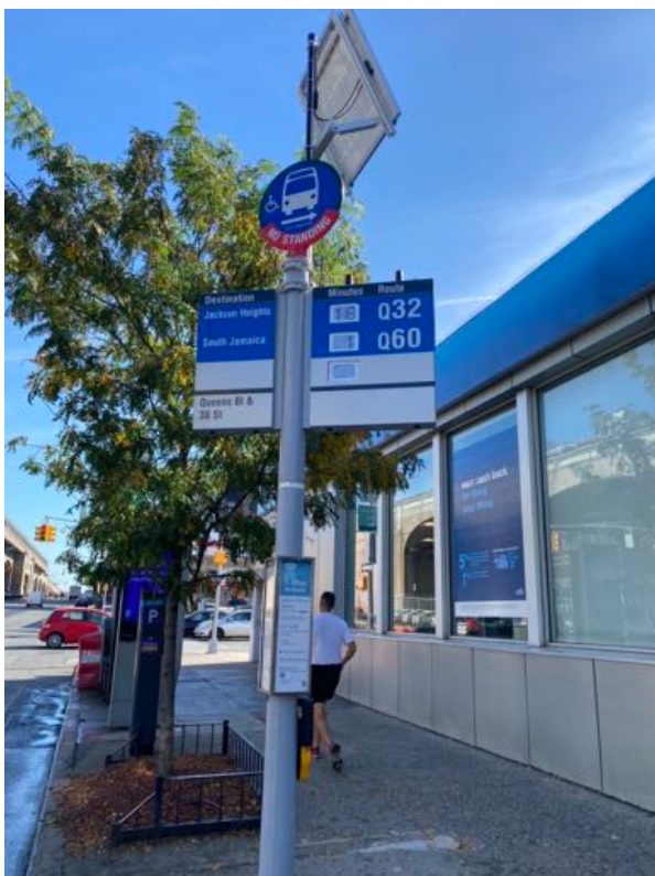
Fig 3. Bus-stop in New York City with 6 electrowetting displays indicating the time to arrival for the next bus. The bus-stop works off-grid and is powered by a solar panel. The electrowetting display has a 7x11 pixel architecture using a direct drive approach with pixels of 10 mm pitch. Photo courtesy of Traffic Systems Inc. and Daktronics.
