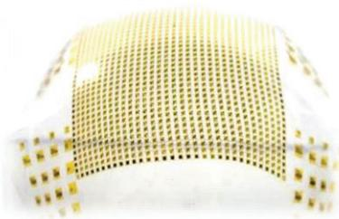
Fig. 9. Photograph of developed dome-shaped stretchable TFT array [11].
