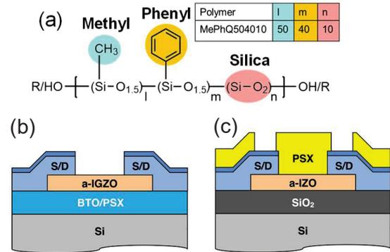
**Fig. 1** (a) PSX structure (b) a-IGZO TFT with BTO/PSX gate insulator (c) a-IZO TFT with PSX passivation
