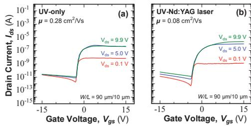
**Fig. 6** Transfer characteristics of fully solution-processed a-IZO TFT on flexible substrates
