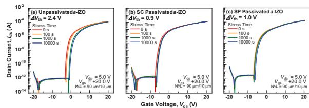
**Fig. 3** Evolution of transfer characteristics of solution processed a-IZO TFT with (a) no passivation (b) spin-coated and (c) spray-coated Fluorinated PSX after PBS stress of 10000 s
