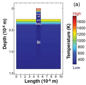
**Fig. 5** 2D multiphysics simulation of laser-induced heating of fully-solution processed TFT.
