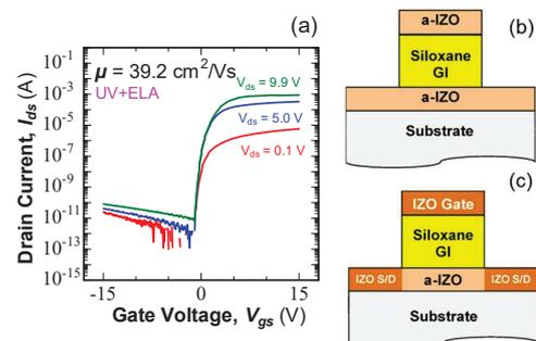
**Fig. 4** (a) Transfer characteristics of fully solution-processed a-IZO TFT. Structure of fully-solution processed TFT (b) before and (c) after electrode activation with either UV, laser irradiation, or plasma process
