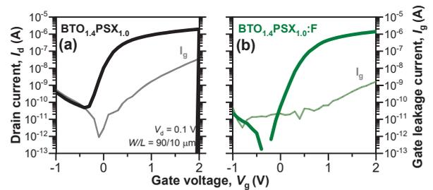
**Fig. 2** Transfer characteristics and gate leakage current of a-IGZO TFT with (a) BTO<sub>1.4</sub>PSX<sub>1.0</sub> and (b) fluorinated BTO<sub>1.0</sub>PSX<sub>1.0</sub>
