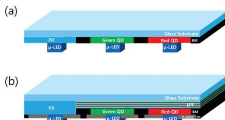
Fig.1 The schematic configuration of GaN based micro-LED structure with (a)conventional QD structure and (b)enhanced QD structure
