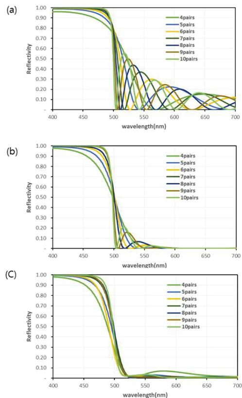
Fig.3 The Reflectance Spectra of (a) [LH]n stack, (b) [(1/2H)L(1/2H)]n stack, (c) [(1/2H)L(1/2H)]n modulated stack
