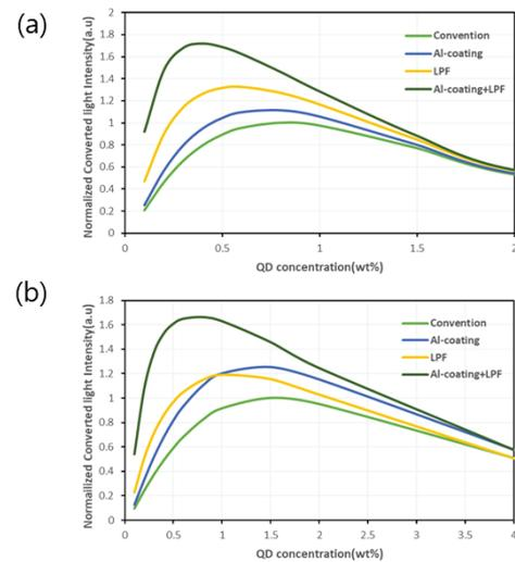
**Fig.5** Intensity of converted light between 0.1wt% to 4wt% QD concentration at 7 pairs LPF structure prepared with and without al-coating and LPF for (a) red QD and (b) Green QD
