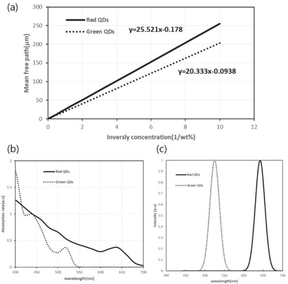
Fig.2 QD nanostructure's optical property: (a) the linear relationship between inverse concentration and MFP, (b) absorption spectra. (c) emission spectra
