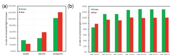
**Fig.4** Color Conversion Enhanced rate for 0.4wt% red QD and 0.8wt% Green QD concentration (a) at each pairs LPF with al-coating, (b) at 7 pairs LPF structure prepared with and without al-coating and LPF
