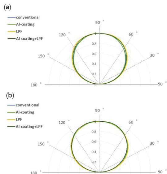
**Fig.6** Normalized relative radiant intensity prepared with and without al-coating and 7 pairs LPF for (a) 0.4wt% red QD and (b) 0.8wt% Green QD concentration
