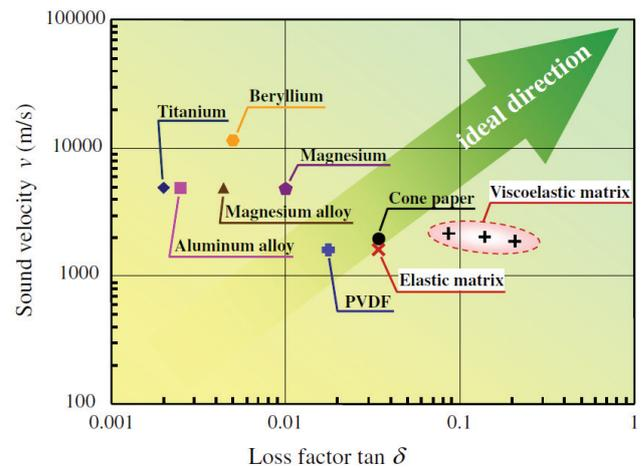
Fig. 4 Acoustic properties (sound velocity and loss factor) of various speaker diaphragms including the electro-acoustic transducers prepared in this study.
