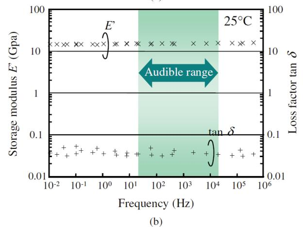
Fig. 3 Rheological properties of the samples: (a) viscoelastic matrix and (b) elastic matrix.
