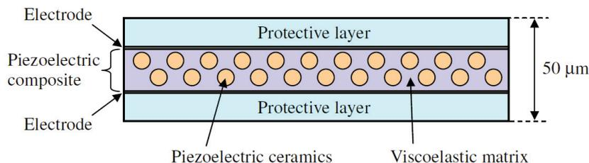
Fig. 1 Schematic of a composite-based electro-acoustic transducer prepared in this study.
