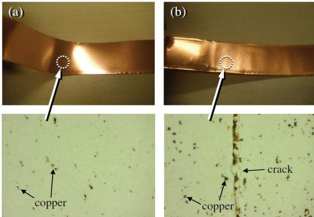
Fig. 2 Appearances of the samples subjected to the roll / unroll test: (a) viscoelastic matrix and (b) elastic matrix.
