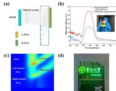
**Fig. 7 (a) PVG-based polarization multiplexing waveguide in-coupling scheme for OLED image sources, (b) Diffraction efficiency spectra and the insert is PVG-based waveguide sample, (c) Simulated results for the PVG-based polarization multiplexing used as an in-coupled grating, (d) Photograph of output images from the OLED image source.**
