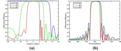
**Fig. 3 (a) Angular and (b) wavelength response of the PVG. The diffraction angles are 20°, 40° and 60° in the RCWA model.**
