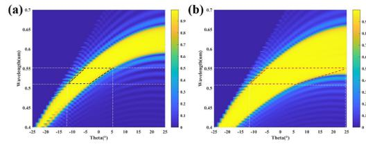
**Fig. 6 Diffraction efficiency distribution of (a) single-layer PVG and (b) stacking-layer PVG at different incident angle and wavelength.**
