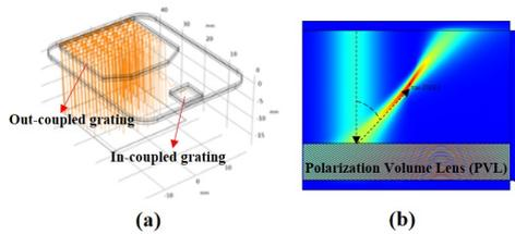
**Fig. 8 The principle scheme of (a) 2D EPE and (b) PVL.**
