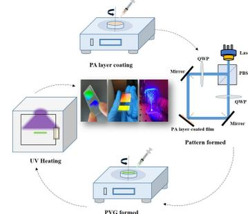
**Fig. 1 The preparation process schematic of PVG.**
