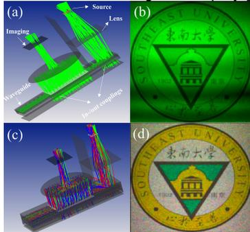
**Fig. 5 One-dimensional expansion waveguide configuration model in ZEMAX. (a) Single-layer waveguide with green source at 532nm, (b) Simulation results of the retina, (c) Three-layers waveguide with full color, (d) Full-color image output.**
