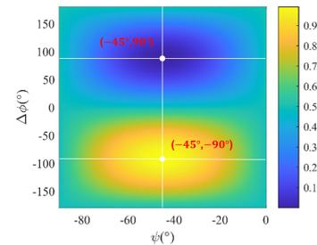
**Fig. 4 The diffraction efficiency of PVG with different incident polarization states.**
