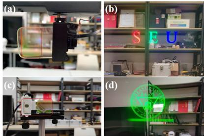
**Fig. 9 (a) Full-color 1D EPE demo with Lcos projector, (b) Full-color output image, (c) 2D EPE with DLP projector, (d) Monochrome output image.**
