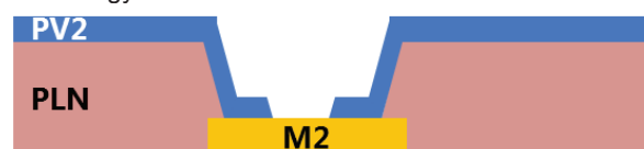
(a) The design structure of PV hole in the PLN layer
