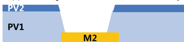
(b) The design structure of PV hole in the PV1 layer
