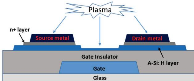
Figure 3. The schematic diagram of the plasma treatment before the deposition of the passivation layer
