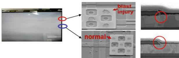
Figure 2. SEM/FIB analysis pictures of undercut
