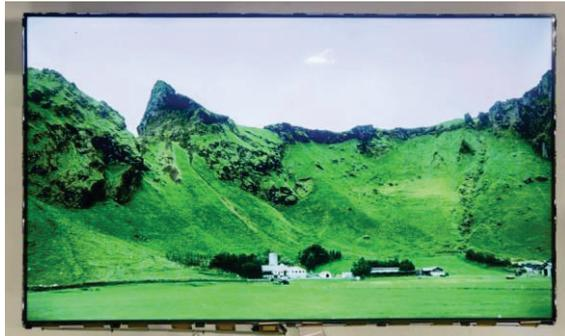
Figure 7. 43DRD 60Hz TFT-LCD panel with the Cu process using 4-mask a-Si TFT
