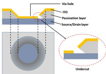
Figure1. The schematic diagram of via hole and the phenomenon of undercut.
