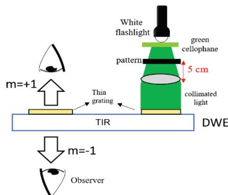
**Fig. 1 The schematic diagram of AR display device compose a pair of thin grating.**
