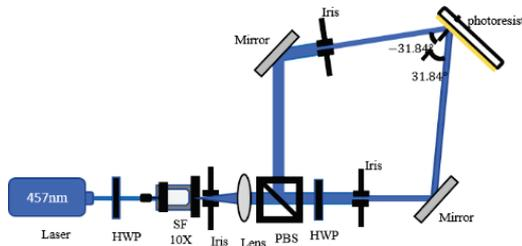
**Fig. 2 The recorded system of DWE. HWP: half-wave plate; PBS: polarized beam splitter; SF: spatial filter**
