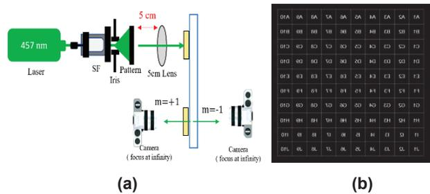
**Fig.4 The observation with LASER backlight by (a) the experimental setup with (b) the target pattern**
