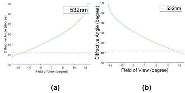
**Fig. 3 The relation between diffractive angle and FOV with  $532\text{ nm}$  wavelength backlight by (a) +1 order of diffraction (b) -1 order of diffraction**
