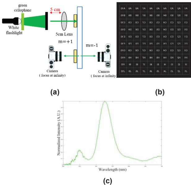
**Fig. 6 The observation with LED backlight by (a) the experimental setup (b) the target pattern (c) the spectrum of LED with green cellophane**
