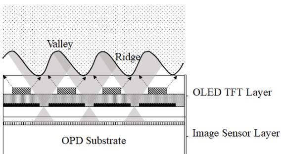
Fig. 1 FOD principle.
