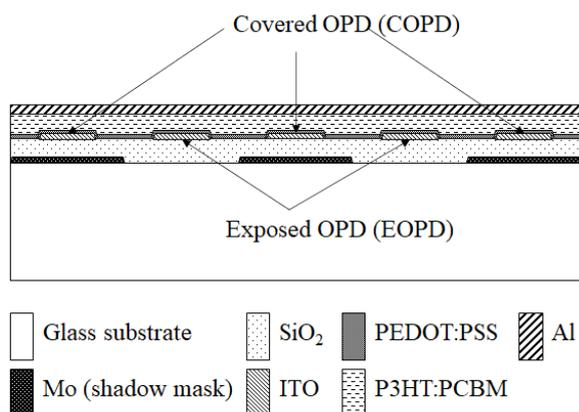
**Fig. 3 Interdigitated electrodes (IDEs) OPDs.**
