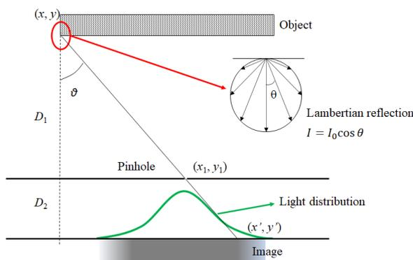
Fig. 2 Pinhole mechanism.
