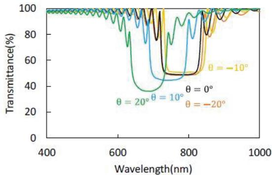
**Fig. 2 FDTD calculated transmission spectra of patterned cholesteric liquid crystal for some incident angles.**
