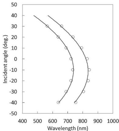
**Fig. 3 Angular dependence of short and long wavelength edges of selective reflection from patterned cholesteric liquid crystal.**
