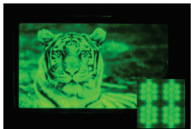
Figure 9: Display samples made with self-aligned process..
